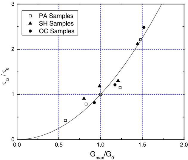
Fig. 1. Relationship between  $G_{max}/G_0$  and  $\tau_{15}/\tau_0$  for PA, SH and OC samples from Hangzhou under the same confining stress (100 kPa).
