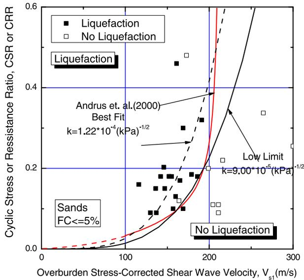
Fig. 8. Correlation curves between CRR and  $V_{sl}$  for sands with lower fines content.
