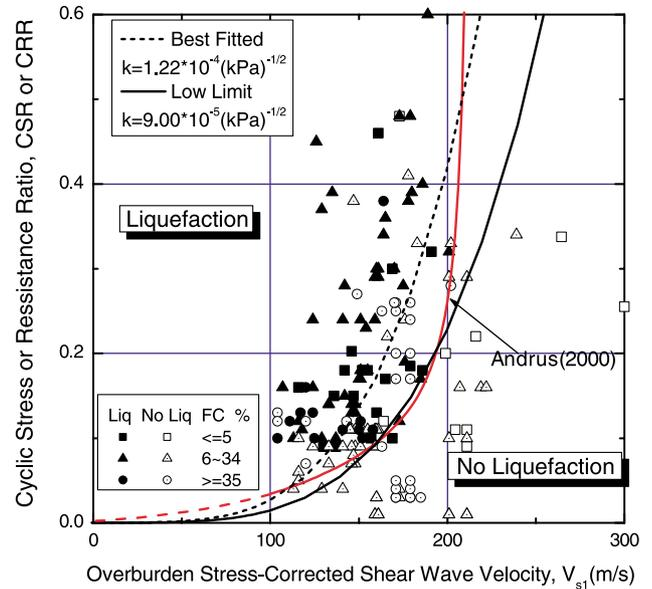
Fig. 9. Correlation curves between CRR and  $V_{sl}$  for sands with different fines content.
