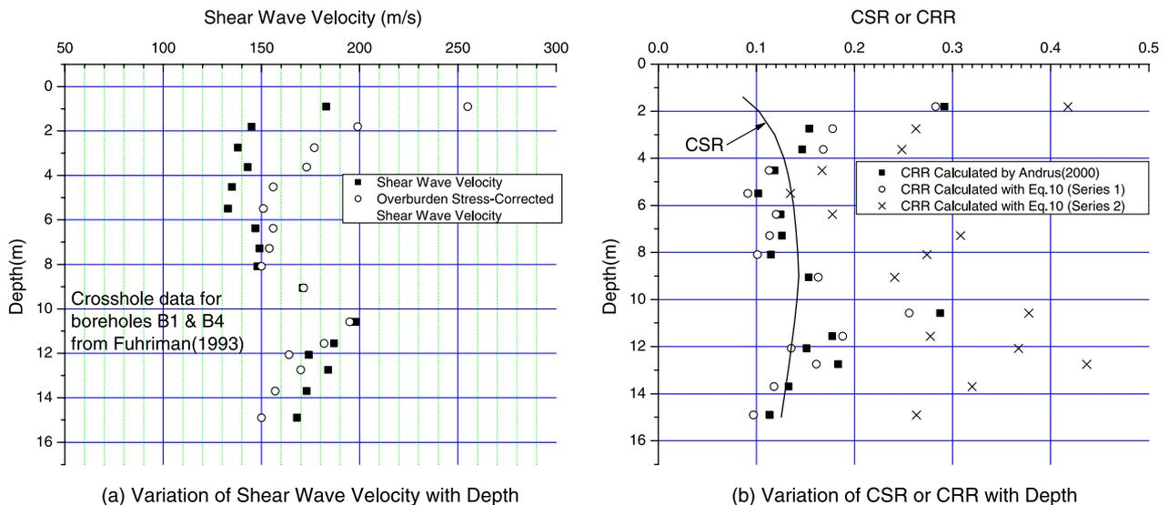
Fig. 11. Comparison of the procedures presented in this paper and Andrus [1] when applied to TI fire station.
