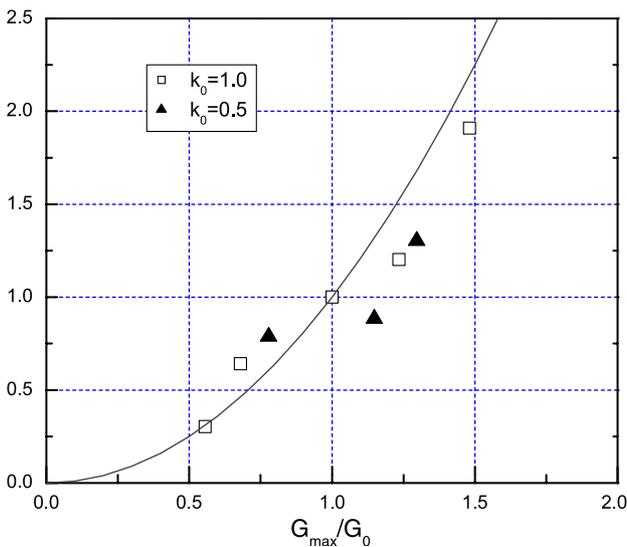
Fig. 2. Relationship between  $G_{max}/G_0$  and  $\tau_{15}/\tau_0$  for PA samples with the same relative density.
